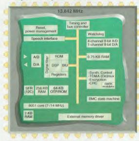
Forming the core of Philips's two-chip DECT solution are the ABC chip that handles ADPCM codec, burst-mode control, and microcontroller functions. The system converts the 1.9-GHz antenna-input signal into two IF signals centered around zero (known as "zero IF chip"). This signal goes to the IF baseband receiver, which converts the analog signal generated by the frontend receiver into the data stream required by the burst-mode controller.
